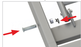
8.2.5 Clevis pin, spacer, and R clip fitting
